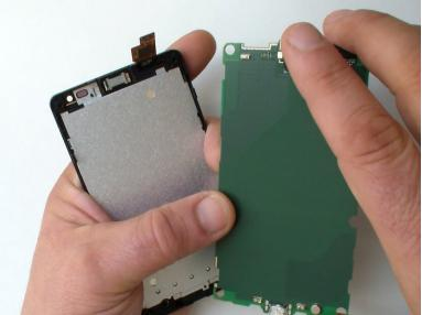
• This is the logic board / main board - a front and rear view.
