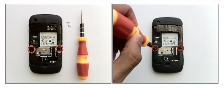
• Remove the two Torx T6 screws to the left and right of the battery.
