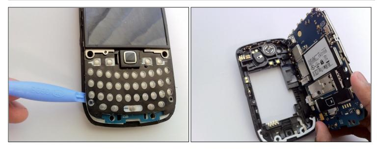
• Using a plastic opening tool, gently pry the motherboard assembly from the device's frame.
