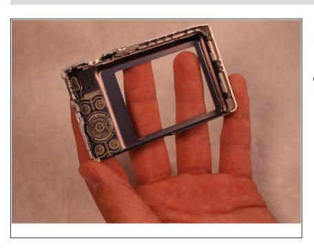
Take the rear panel of the device in the palm of your hand with the buttons facing downward.
