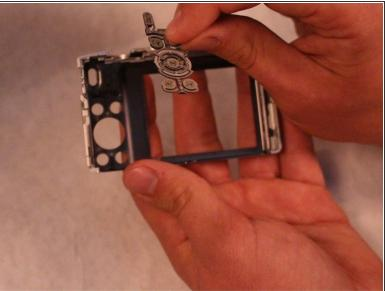
Now, take the hand that was previously holding the pry tool, and finish pulling off the rear function buttons.
