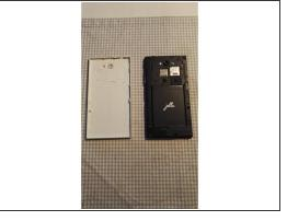
Remove the back cover by pulling up from the bottom right hand corner. Remove the bottom first and then the sides.
