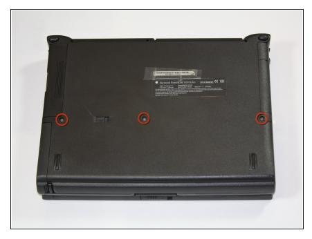
Turn the laptop over and remove the three T8 torx screws from the bottom panel.
