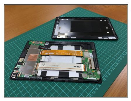
The back case didn't use any screw or glue. The back case only use tenons to stick with front case. It's not hard to take apart.
