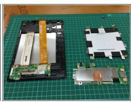
(i) There are three big parts in tablet-- upside circuit board, battery and downside circuit board. Base on my experience, upside circuit board has more important IC chips than downside board.
