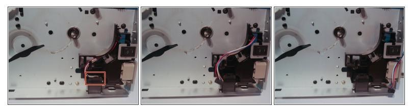
Disconnect the cable to the tray connector and route it through the hole in the chassis.
