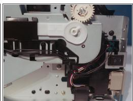
Remove the fan cable from the cable guide.
