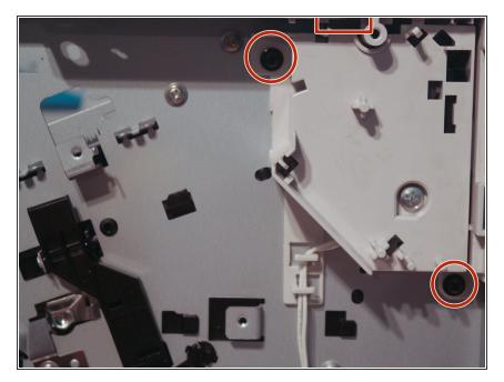
Remove 3 screws from the safety interlock assembly (one on top) and remove it from the printer.
