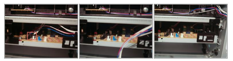
Disconnect 2 cables from the main board and route them through the cable guide.
