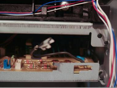
Use needle nose pliers to disconnect the high voltage wire from the fuser.
