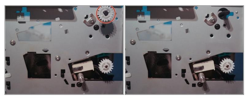
Remove the fuser gear by pushing in on the tab with a metal spudger.
