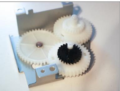
Remove 3 screws holding the duplexer gears to the printer and remove the gears.
