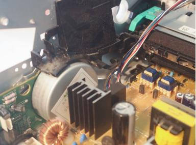
Remove the tray connector and motor cables from the cable guide.
