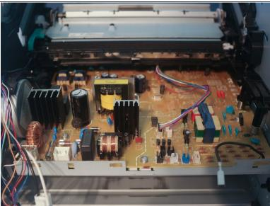
Remove the feed plate from over the main board.
