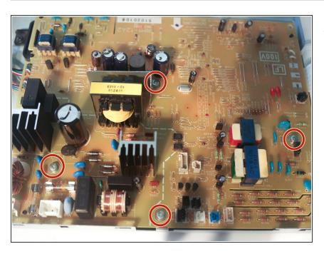
Remove 4 screws on the control board to remove it from its metal plate.
