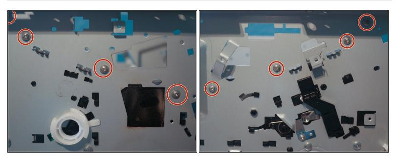
Remove 4 screws from each side of the printer to remove the mainframe.
