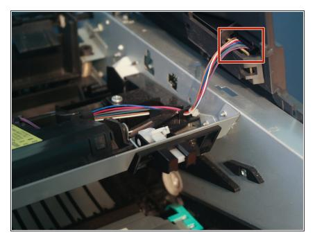
Disconnect the control panel cable and remove the top cover.
