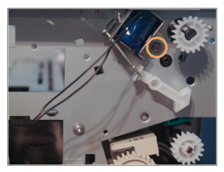
Remove one screw to remove the solenoid from the printer.
