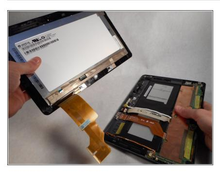
Lift the screen upwards to remove.
