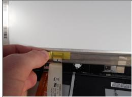
Remove the yellow tape covering the end of the cables.
