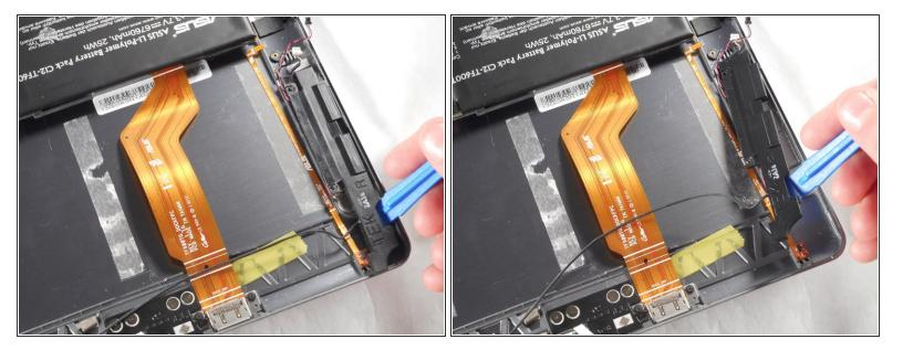
Remove the speaker with the plastic opening tool.
