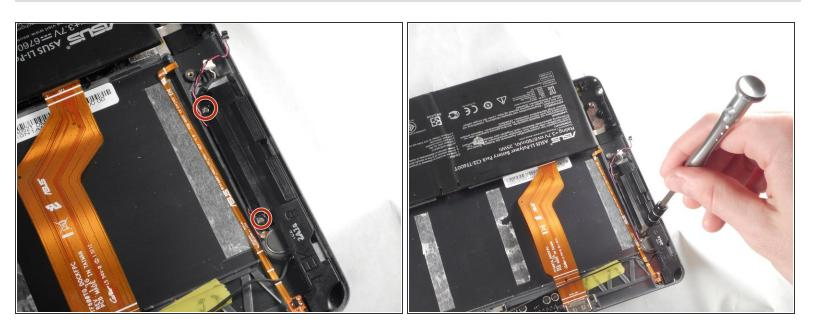
Remove two 0.79 mm #00 screws from the speaker with a Phillips screwdriver size #00.
