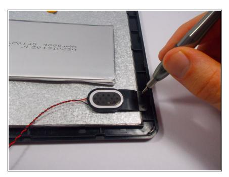
Next you will need to remove the two screws attached to the speaker. If you have a 54 bit Driver Kit use the Philips Head 0 (or PH 0) head to remove the two 4mm screws.
