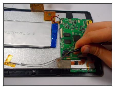
Remove the second layer of tape above camera cable connection gently and remove the cameras from the device.
