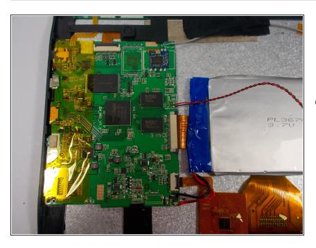
Be sure that all the connections to the motherboard are disconnected.
