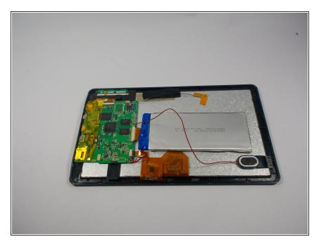
Pry battery up from adhesive. Use a type of adhesive remover. Nail polish remover works well.
