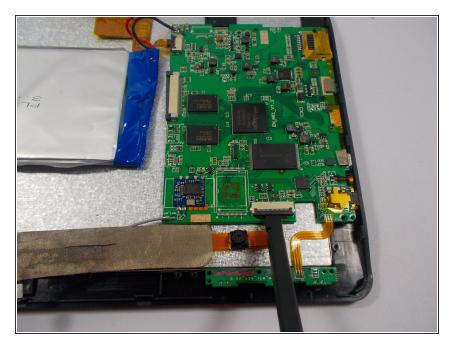
Disconnect the camera from the mother board. Use a spudger and lift the grey latch until it is facing up then pull out the connection for the cameras.
