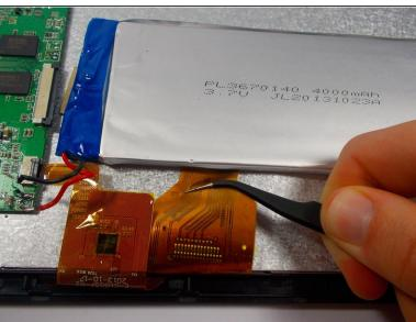
Use a pair of tweezers to grasp the screen/digitizer connection gently and remove each accordingly.
