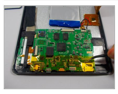
Grasp the EDC tape with your tweezers and lift it off gently from the motherboard and set aside to be reused.
