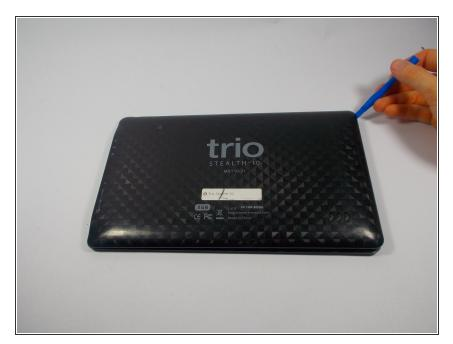
To remove the back panel, you will need to use a plastic opening tool and slowly separate the back panel from the device.
