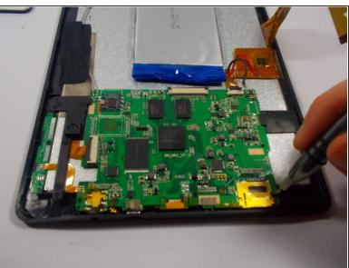
Use a Phillips #0 to unscrew the 4mm screws from the motherboard fixture.
