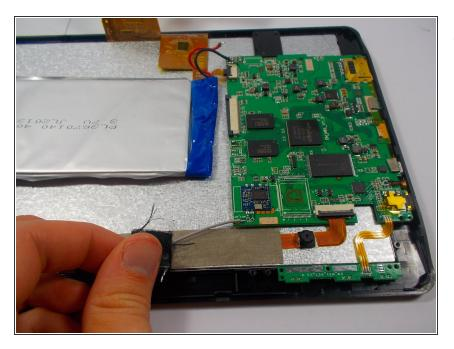
Remove the first layer of tape above camera cable connection slowly.
