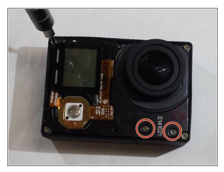
Remove the two screws to remove the riser that is being held in place by the screws.
