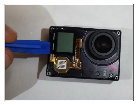
Now, you will need to remove the camera and boards from the black plastic housing. You may use any tool that will do the job. My group found out, if you use the plastic tool to remove the boards and camera, that it would assist you with the removal.
