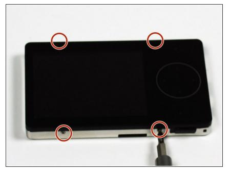
Unscrew the four screws (size: 3.175mm) on the left and right side of the Element Electronics GC-1020 device using the PH#0 screwdriver.
