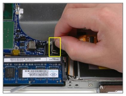
Disconnect the display data cable by pulling up on the black plastic pull-tab. If there is no pull-tab on the top of the connector, it may be helpful to use a spudger to disconnect this connector.
