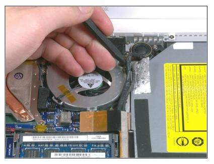
Use a spudger to move the gray display data and black speaker cables to the right. This will reveal a silver screw securing the fan housing to the lower case.
