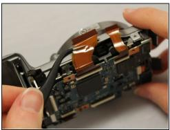
• Locate 3 thick ribbon cables on the bottom, and flip up the white retaining tabs. Pull out the remaining ribbon cables, utilizing <u>tweezers</u>.
