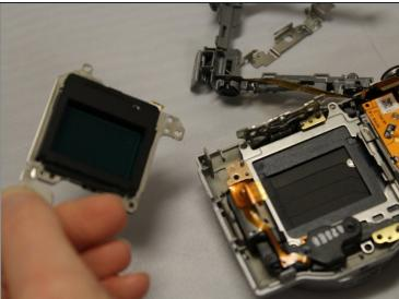
Detach the circuit board from the device.
