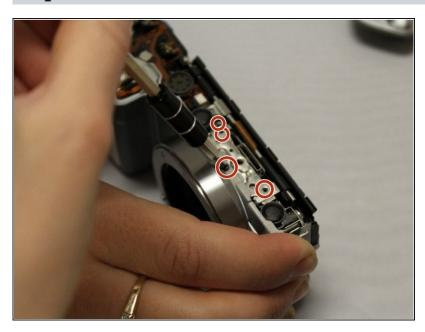
To the right of where you unscrewed the copper screws, unscrew 4 black 1.2 mm Phillips #000 screws.
