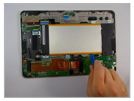
Use plastic opening tool to carefully pry the battery out from frame.
