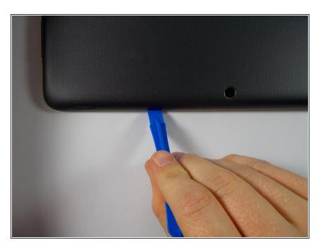
Slide the tool in the gap along all four sides, continually pulling the tool upwards.
