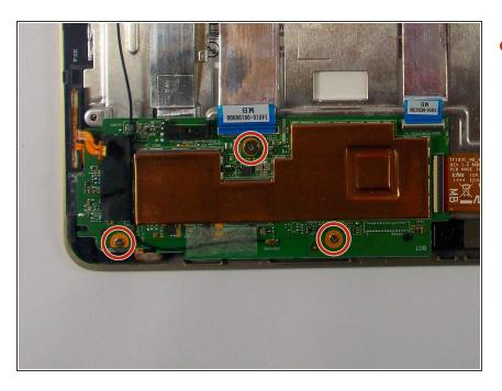
Use the +J000 screwdriver to remove screws (3) from motherboard.
