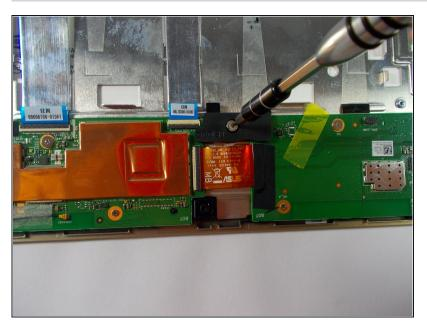
• Use the +J000 screwdriver to unscrew and remove the M2 screw and plastic bracket.
