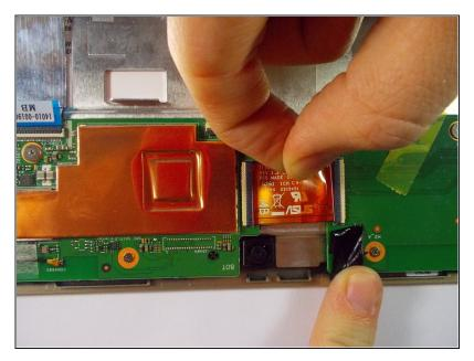
• Remove the black tape from the ribbon cable and separate the cable from the soundboard.
