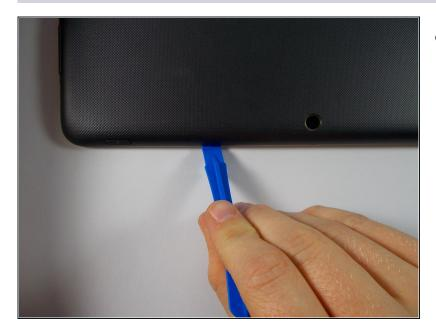
Slide the tool along all four edges of the laptop and continue to pull the tool upwards to fully remove the bottom case from the laptop.
