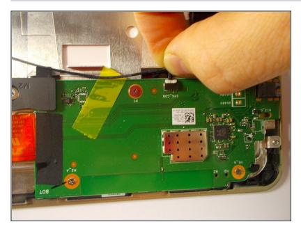
• Remove the tape and unplug the wire that attaches to both speakers from the soundboard.
