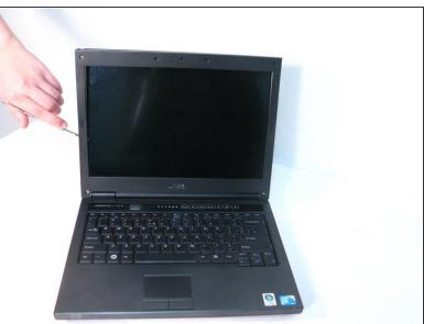
Pop the black plastic panel off with the metal spudger. There are three spots where you should leverage it so that the panel does not break.
