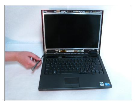
Remove the two screws on the bottom of the computer screen.
