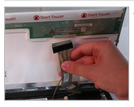
Remove the tape and the LCD plug/connector from the back of the screen.
