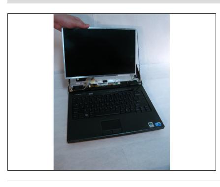
Remove the screen from the metal side frames.
