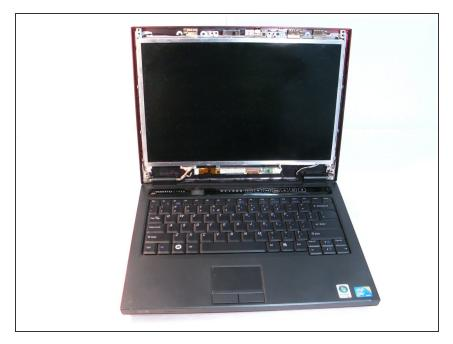
Remove the plug on the bottom of the screen.
