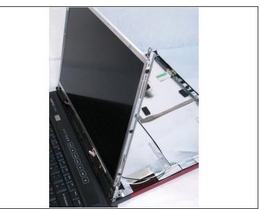
Remove the three screws on the left and right of the screen.
