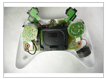
Locate the two 4 mm motherboard screws, shown circled in red, with the J0 screwdriver.
