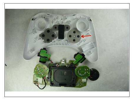
Remove the motherboard and connected components. The rubber pad of the D-Pad is indicated in the image by the red arrow.
