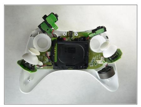
Remove the joysticks and motherboard from the controller's shell.
