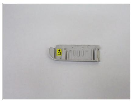
Make sure that the new battery door is groove side up so that the door will slide onto the metal bracket on the device.
