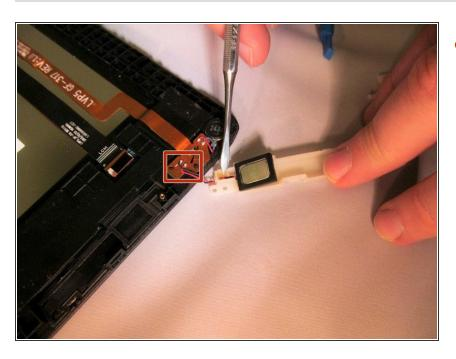
Using a soldering iron, desolder the contacts that connect the speaker wires to the speaker chip.
