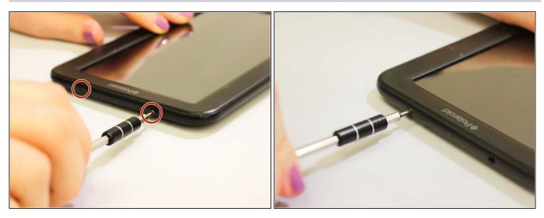
• Remove the two 7 mm screws on the top of the device using a J00 Phillips screwdriver, turning them counterclockwise.
