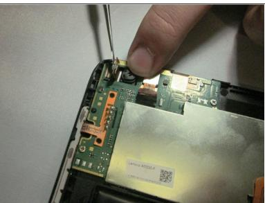
Using a spudger, pry upward on the camera connector to free it from the motherboard.
