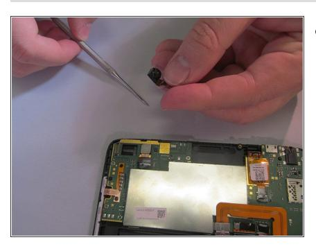
Use tweezers to grasp the camera connector and lift the camera out of its socket.
