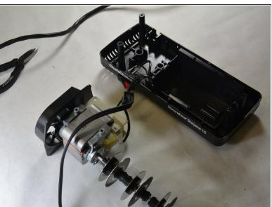
With the outer case removed, firmly grasp the motor-axle attachment and remove it from the base.
