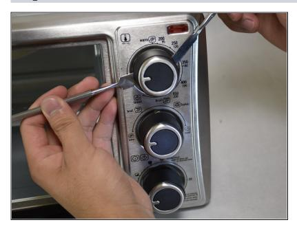
Using two metal spudgers, pry the top control knob directly outward.
