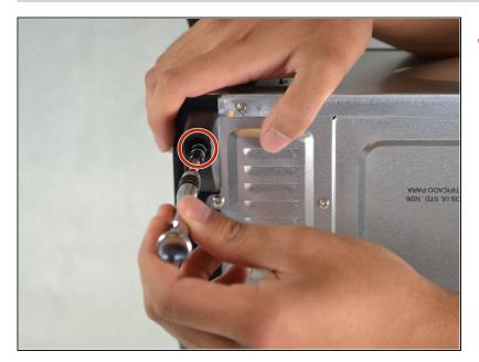
Remove the 11.5 mm screws using a #2 Phillips screwdriver.
