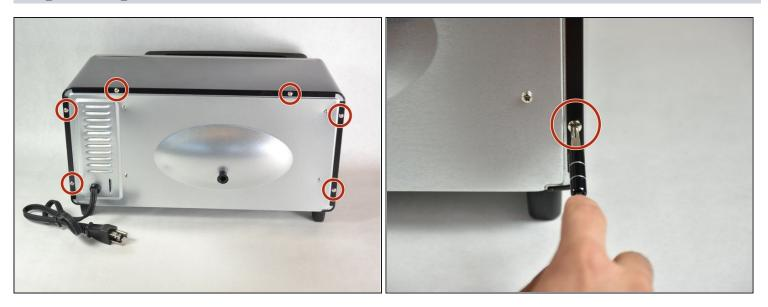
• Remove the six 9.5mm screws on the back panel using a #2 Phillips screwdriver.
