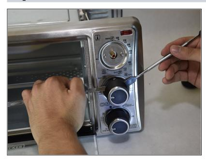
Using the two metal spudgers, pry the middle control knob directly outward.
