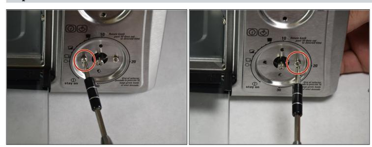
• Remove the two #2 Phillips Head x 5.5mm screws holding the timer controls to the face.
