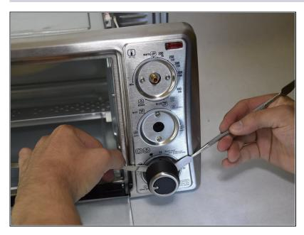
Using the two metal spudgers, pry the bottom control knob directly outward.
