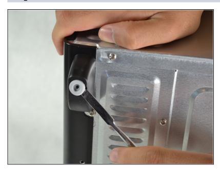
Using the metal spudger, carefully pry out the rubber base on each foot to access the screws.
