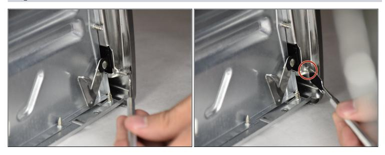
• On the left side, use a metal spudger to push the hinge pin in as far as you can.
