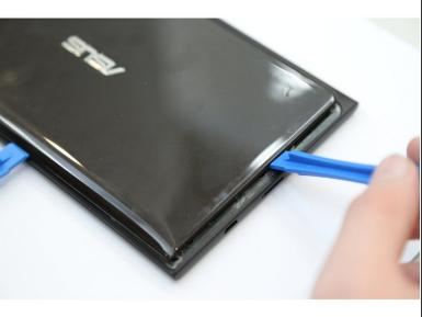
• Make sure your device is turned off. Then with a plastic opening tool, carefully remove the back panel by carefully working your way around the perimeter.
