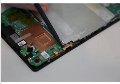
Locate the GPS antenna. Pry off the GPS antenna cable with a spudger.
