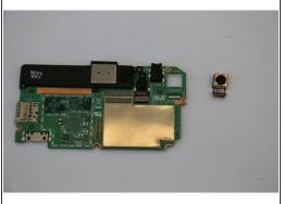
Using tweezers, carefully remove the rear camera connectors and place it to the side.
