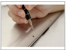
Remove the twelve 3 mm bottom panel screws with a <u>T5 Torx Screwdriver</u>.
