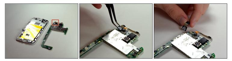
• Use the prying <u>tweezers</u> to remove the front facing camera.
