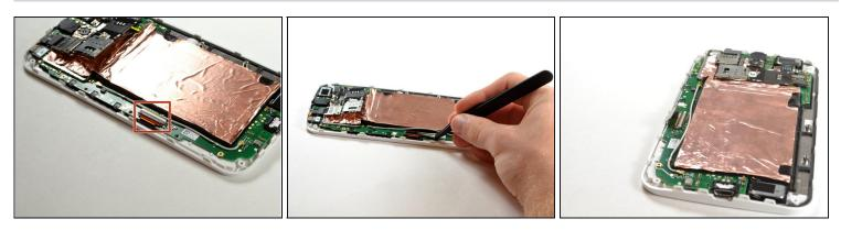
• Remove LCD connector by lifting the black plastic flap.
