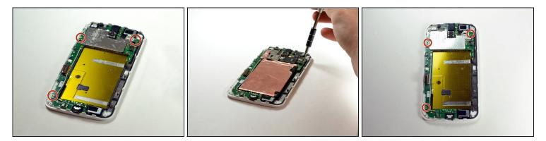
• Using a T5 Torx screwdriver, unscrew the three 2.2 mm screws holding the motherboard in place.
