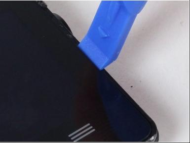
Place the blue plastic opening tool in-between the screen and plastic casing of the watch and slowly pry up one side of the screen.
