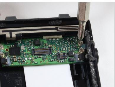
Remove the four 2.4 mm screws with a PH00 Phillips head screwdriver.
