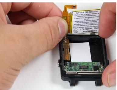
Use a plastic opening pick to gently pry out the battery as shown.
