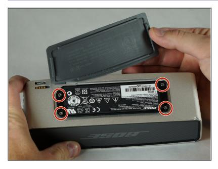
Peel back the rubber battery cover and remove the four circled 6.0 mm screws using a T8 Torx Screwdriver.
