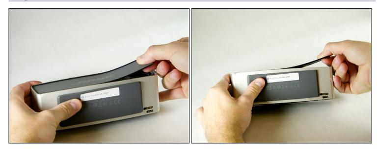
• The grille is attached to the speaker with double sided sticky tape. To remove the grill gently pull upward while keeping tension to the right.
