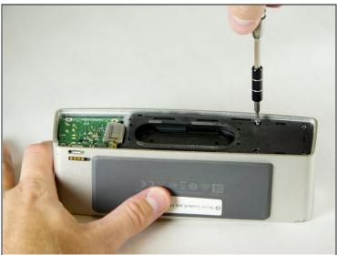
• Remove the four 15.0 mm screws on the left and the four 9.0 mm screws on the right using the T8 Torx Screwdriver.
