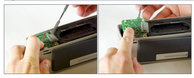
• Remove the circuit board by pushing it with your index finger in the direction shown while using a nylon or metal spudger to lift it up and out of place.
