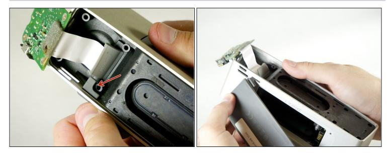
• Carefully pull on the battery cover until the rubber tab slides out of the aluminum casing.
