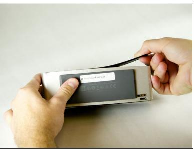
The grille is attached to the speaker with double sided sticky tape. To remove the grill gently pull
