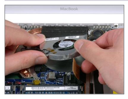
Lift the fan and its attached mounting bracket up and out of the computer, being careful not to rip the black felt tape.
