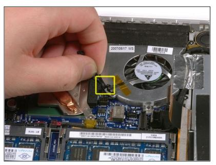
Deroute the fan cable from behind the tab on the left side of the fan.
