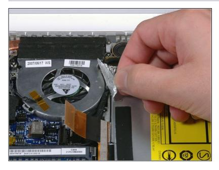
Peel up the silver foil tape between the fan and the optical drive.
