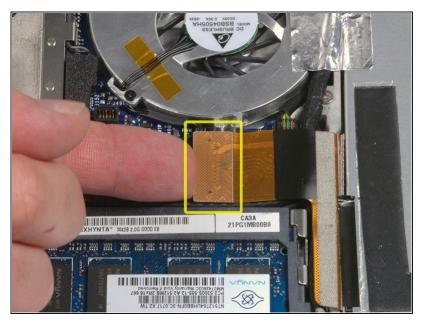
Use a spudger to disconnect the orange optical drive cable from the logic board.
