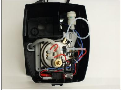
Remove the four 16mm screws with a T20 Screw head.
