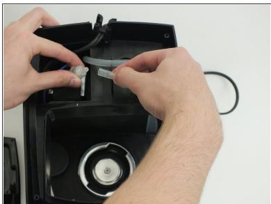
Flip the device and remove one end of the tube from the water reservoir hole.
