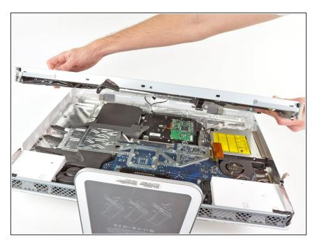
Remove the display assembly from the iMac.
