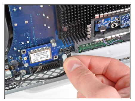
Pull the ambient temperature sensor cable perpendicular to the face of the logic board to disconnect it from its socket.
