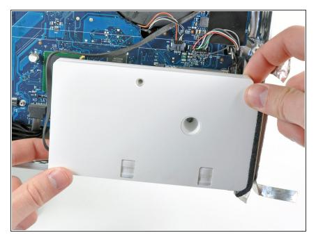
Pull the right speaker away from the logic board and remove it from the iMac.
