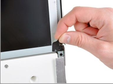
Peel the two highlighted EMI shield tabs off the frame of the LCD.
