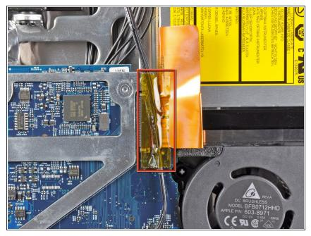
i If necessary, remove the strip of tape covering the optical drive connector.
