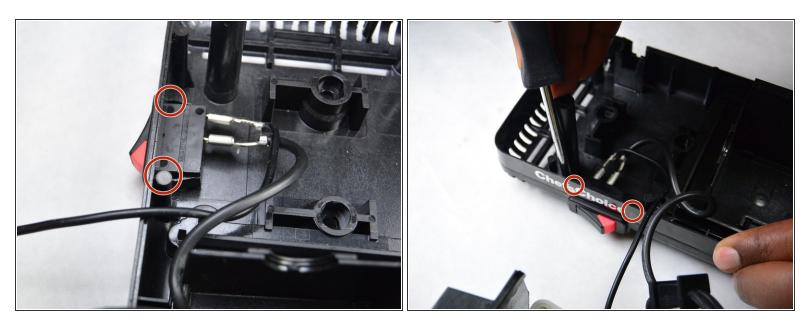
• Using a screw driver, unclip the edges of the switch by pushing them inwards and nudging the switch out of the plastic casing. You will hear a click when the edges unhook from the casing.
