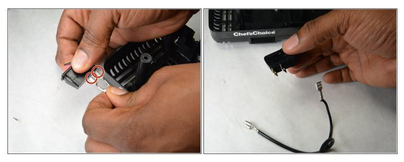
• Remove the spade connectors from the switch by pulling only on the connector, not the wire.
