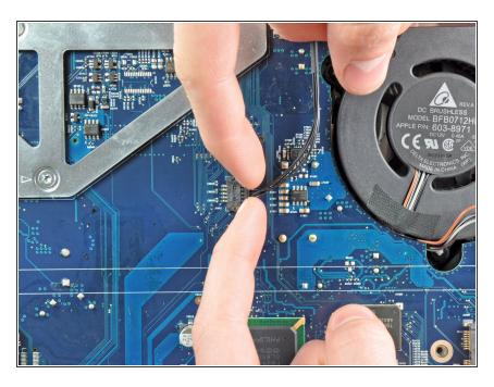
Pull the optical drive thermal sensor connector toward the right side of the iMac to disconnect it from its socket.
