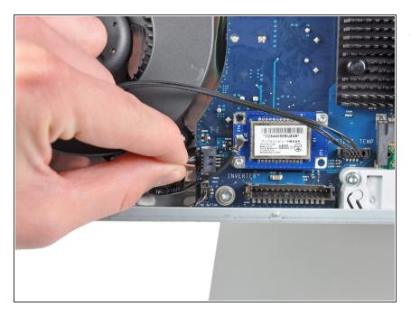
Pull the CPU fan connector toward the left edge of the iMac to disconnect it from the logic board.
