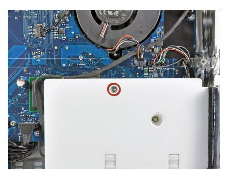
Remove the 26 mm T10 Torx screw securing the right speaker to the iMac.
