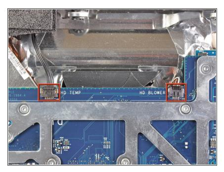
Disconnect the hard drive thermal sensor and hard drive fan cables from the logic board by pulling their connectors toward the top edge of the iMac.
