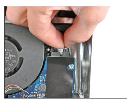
Pull the left speaker connector toward the top edge of the iMac to disconnect it from the logic board.
