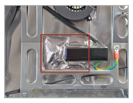
Peel the three pieces of aluminum tape away from the body of the AC inlet to reveal all three of its mounting screws.
