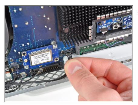
Pull the ambient temperature sensor cable perpendicular to the face of the logic board to disconnect it from its socket.
