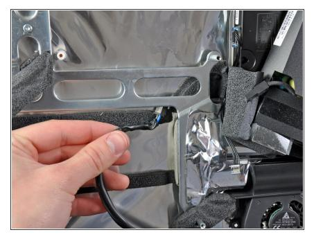
De-route the AC inlet cable from underneath the metal framework attached to the rear case.
