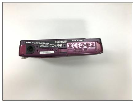
Place the Nikon Coolpix upside down so that the on/off button is facing the floor and the camera information is facing you
