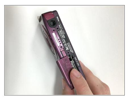
Slide the battery cover away from the camera to reveal the location of the battery
