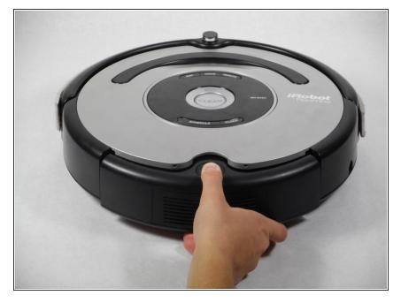
Press the black circular button on the back end of the Roomba and pull the bin out towards you to remove the vacuum bin.
