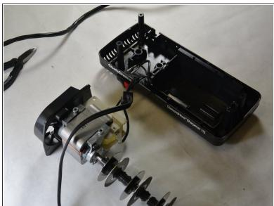
Carefully lift the entire motor assembly out of the case.
