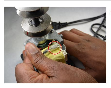
Disconnect the spade connector on the motor by pulling only on the connector, not the cord.
