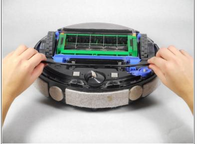
Lift the thin top cover that holds the bumper in place.
