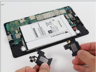
• Use a spudger to pry the uper speaker up and away from the device.
