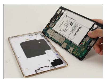
Remove the back cover after the entire rim is disconnected.
