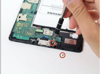
• Remove the two 2 mm Phillips #000 securing the headphone jack.
