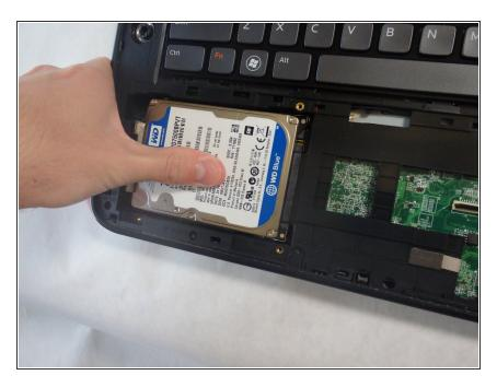
Slide the Hard Drive away from the mouse pad to disconnect/unplug it.
