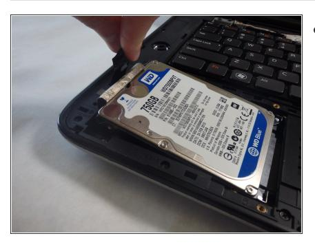
Pull the tab up and out to remove the Hard Drive.
