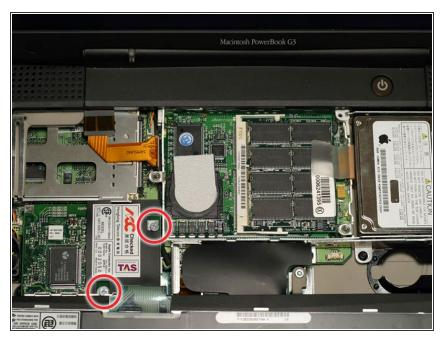
• Remove the two silver Phillips screws from the modem.
