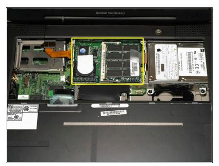
• Use a spudger, the tips of your fingers, or a flat non-metal tool to pry up the processor's right side.
