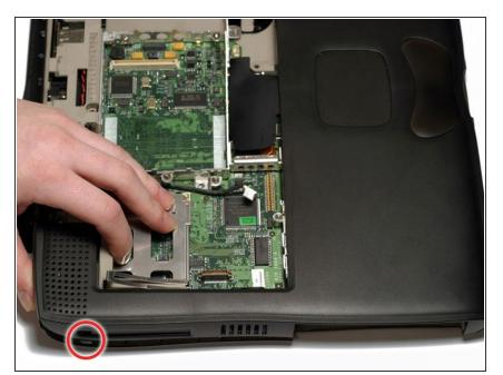
• The PC card eject button on the laptop's left side prevents the upper casing from lifting up. In order to bypass the button, push it in far enough so that you can pull the upper casing's left side out and up beyond the button.
