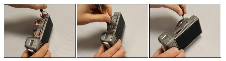
• Unscrew the 3 silver 1.2 mm Phillips #000 screws from the bottom of the camera.
