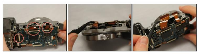
• Locate 3 thick ribbon cables on the bottom, and flip up the white retaining tabs. Pull out the remaining ribbon cables, utilizing <u>tweezers</u>.
