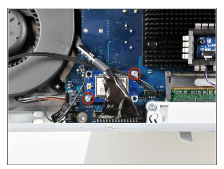
Remove the two T6 Torx screws securing the Bluetooth board to the logic board.
