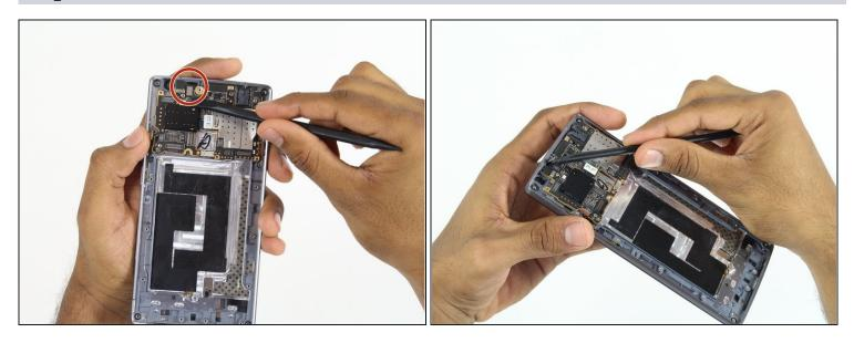
Use the spudger tool to pry up the connection at the top of the motherboard.
