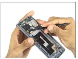
• Use the spudger tool to pry off the 2 connections at the bottom-left of the motherboard.
