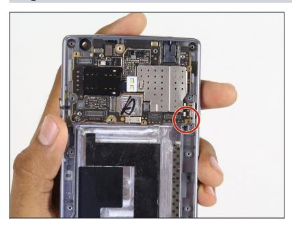
Use the screwdriver to unscrew the screw fastened at the bottom right of the motherboard.
