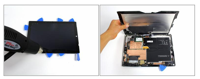
Lift the screen up carefully so that no wires are torn.
