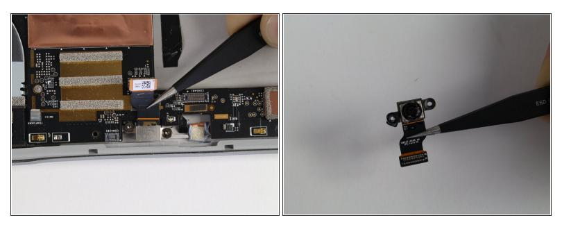
• Remove the rear camera with the tweezers.
