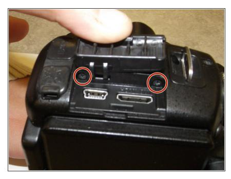
While you are on the left side of the camera, lift the HDMI / USB cover and remove the two screws that are hidden.
