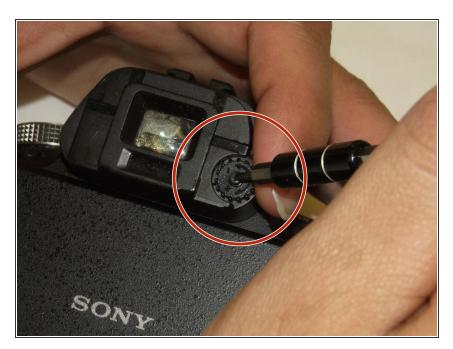
Start by removing the focusing knob on the back of the camera.
