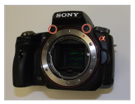
Remove the two screws immediately below the flash. These screws are located on the face of the camera.
