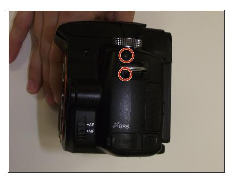
Remove two screws from the left hand side of the camera.
