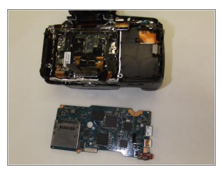
Once the motherboard has been completely unplugged and removed, it can be replaced and reassembled in reverse order.
