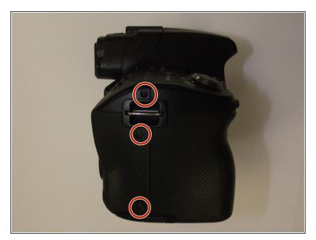
Remove three screws from the right side of the camera.
