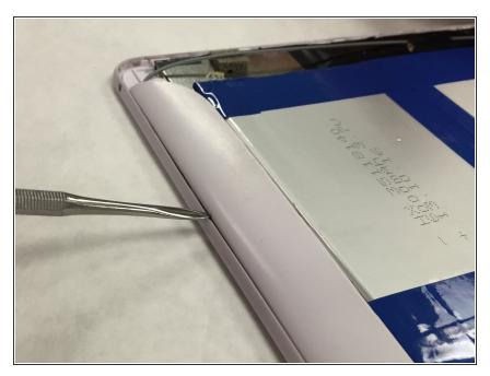
• Use a prying tool to remove the plastic piece off of the antenna component.
