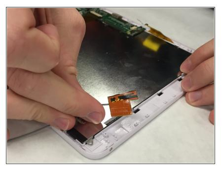
Once all of the adhesive tape has been removed. Pull out the antenna component.
