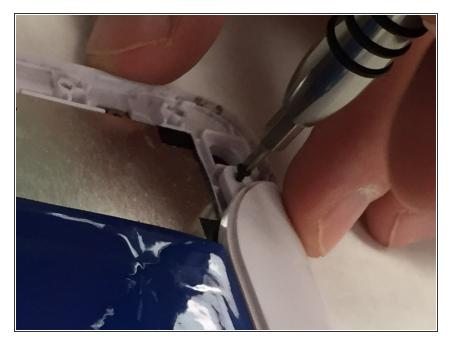
• Remove the two screws holding the antenna cover in place.
