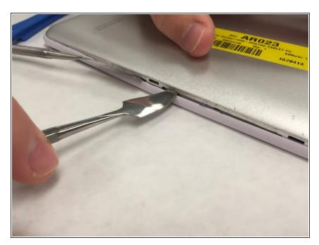
• Remove the back panel of the device.
