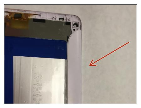
• Identify the antenna cover on the top of the device.
