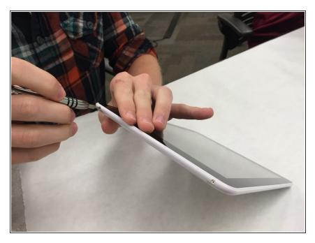
• First step is to remove screws from top and bottom of device.
