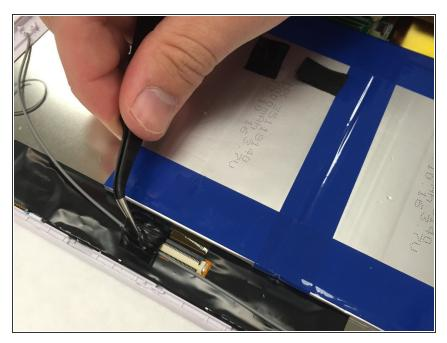
• Remove all of the adhesive tape pieces off of the antenna cable.
