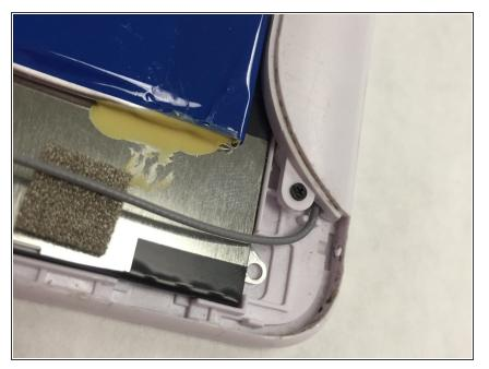
Identify the antenna component as the gray cable that comes out of the plastic cover.
