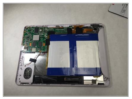
• Upon removing the back panel, place the device screen down on the table.
