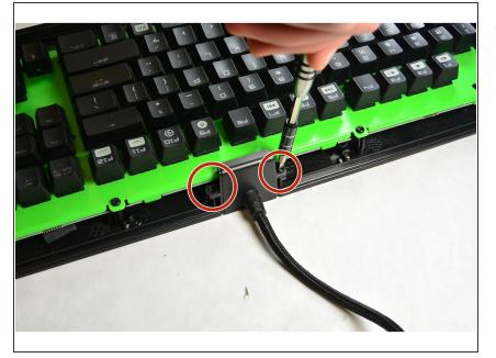
Find where the cable enters the back of the keyboard. There are two screws on either side of the tab holding the cable in. Once removed, the tab should slide out of the keyboard.
