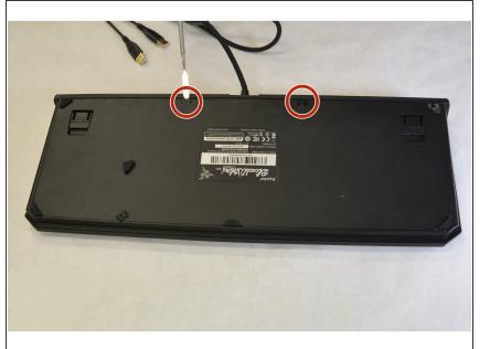
There are two tabs on both sides of where the cable enters the back of the keyboard. Use the metal spudgers to gently pull up the tabs. These are circled in red on the picture.
