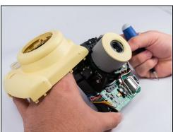
⚠ Use the plastic opening tools and spudger to safely remove the front shell casing.
