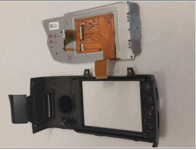
Remove six 5 mm x 4mm head screws, then remove the metal plate from the plastic camera backing.
